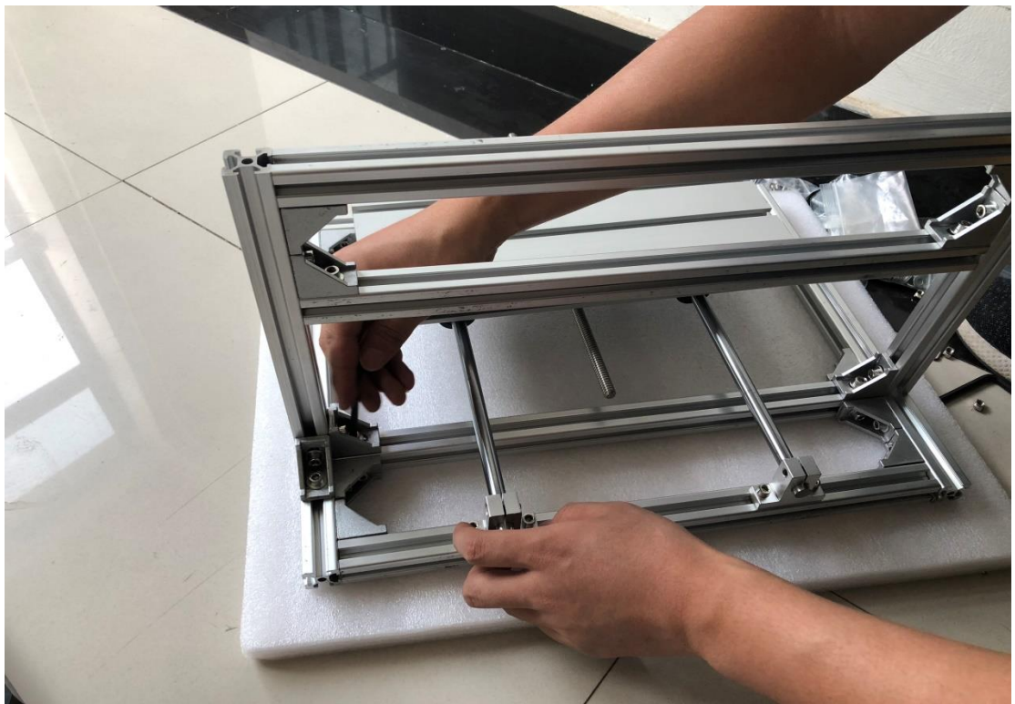
3. Adding the additional brace - a 3D printed part.
